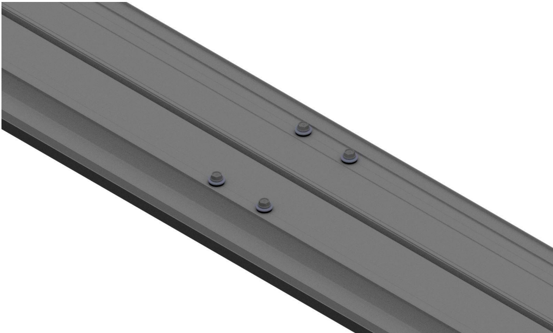
Fig. 68 Join the base rails together and screw in 2 more sheet-metal screws
