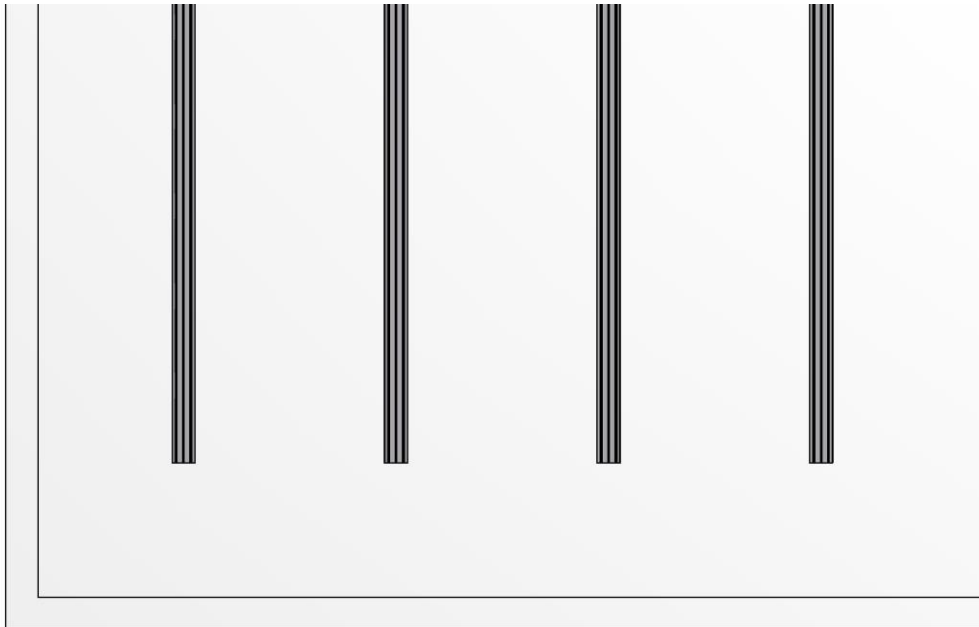
Fig. 20 Align the base rails so that they are parallel and vertical.
